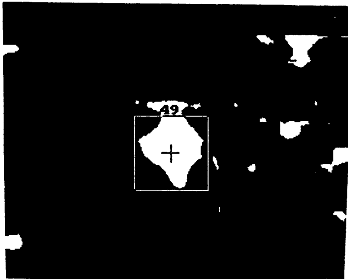
(b) Stitched Specimen # STSI-15: C-Scan Damage Area = 446 mm 2
