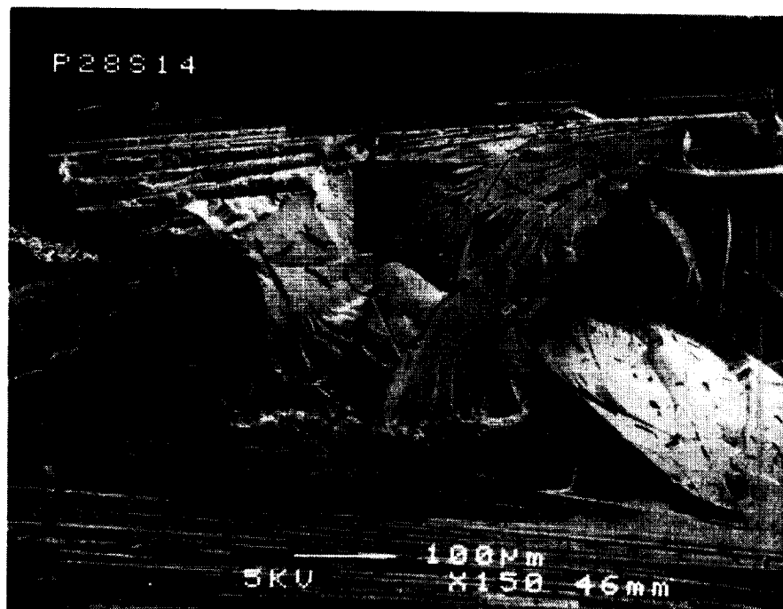
Figure 3-15: Matrix in the adjoining area of the Glass -750 stitch appears "ploughed"
