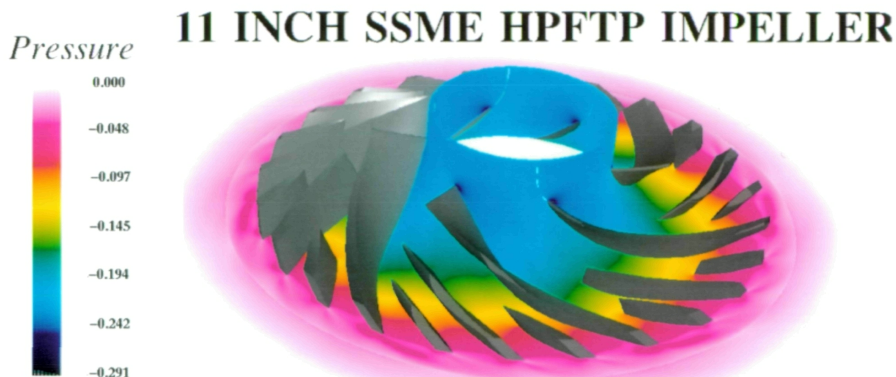
Figure 1 : Hub surface colored by static pressure
