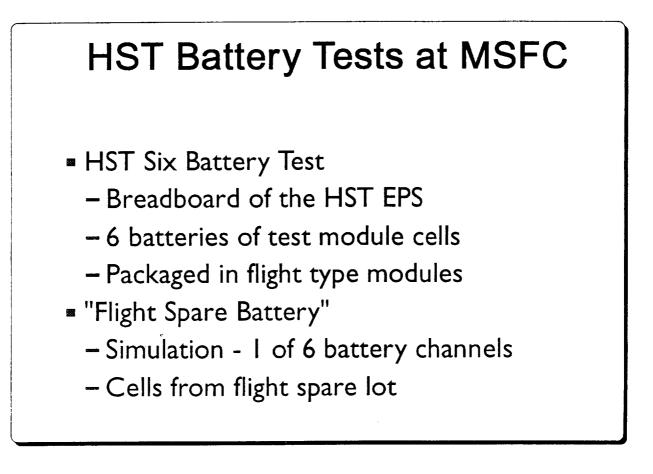
The <u>HST Ni-H2 Six Battery Test</u> is a breadboard of the HST EPS. The batteries in the test are composed of test module cells and packaged into 3 battery modules identical to the flight modules. This test is the HST EPS Testbed.
