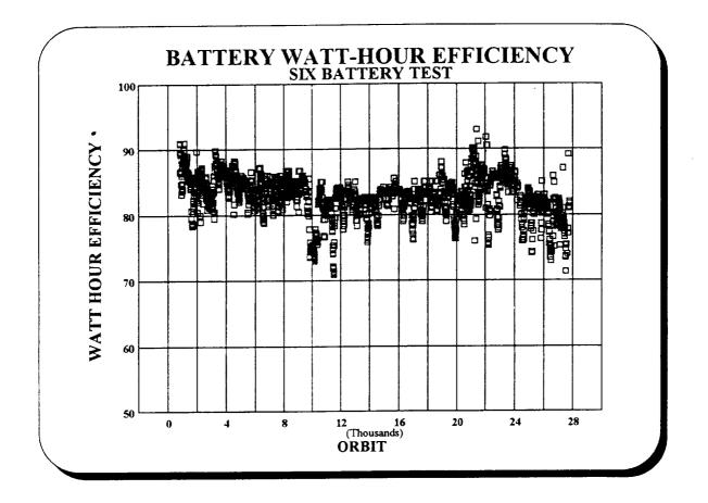
This plot shows the average battery watt-hour efficiency over the life of the HST Ni-H2 Six Battery test. The batteries cycled with a step to trickle charge scheme and charged to 1.5 v/cell for the first 20k orbits. After orbit 20k the charge scheme was changed to hardware control (essentially a taper charge) and the charge voltage was lowered to 1.49 v/cell. The watt-hout efficiency of the HST Ni-H2 cells has varied from about 77 to 85%.
