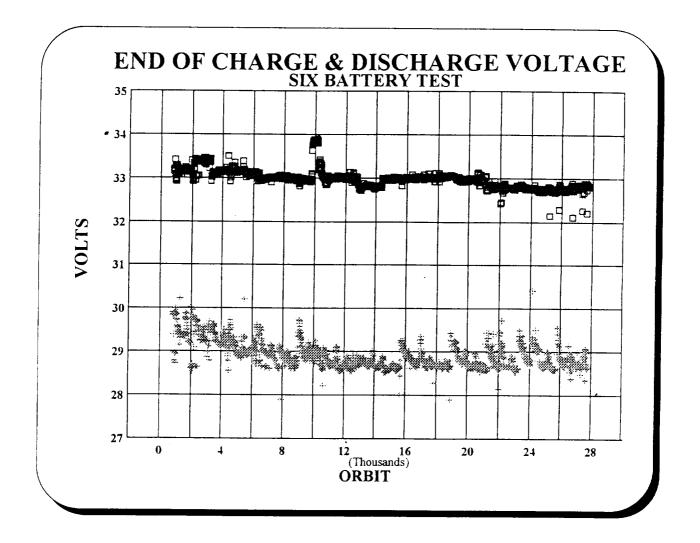
This plot shows the end of charge and end of discharge voltages over the life of the Six Battery Test. The end of charge voltage tracks the different charge levels that have been used and the end of discharge voltages track the general state of health of the batteries. Even though the end of discharge voltages have essentially stabilized, a gradual decline over the life of the batteries is to be expected.
