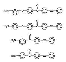
The phenylethynyl group is the functionality which reacts at elevated temperatures, while the amine group allows the compound to be incorporated into any system which reacts with an amine. Any compound having the following general structural formula can also be used as an endcapping agent
