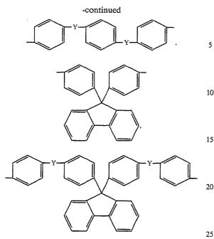
wherein Y=nil, O, S, C=O, SO<sub>2</sub>, CH<sub>2</sub>, C(CH<sub>3</sub>)<sub>2</sub>, C(CF<sub>3</sub>)<sub>2</sub> etc., and mixtures thereof.
