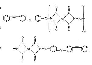
wherein Ar is any diamine moiety Ar' is any dianhydride moiety, x is a member selected from the group consisting of: a bond, a meta-substituted phenoxy group and a para-substituted phenoxy group: y is a member
