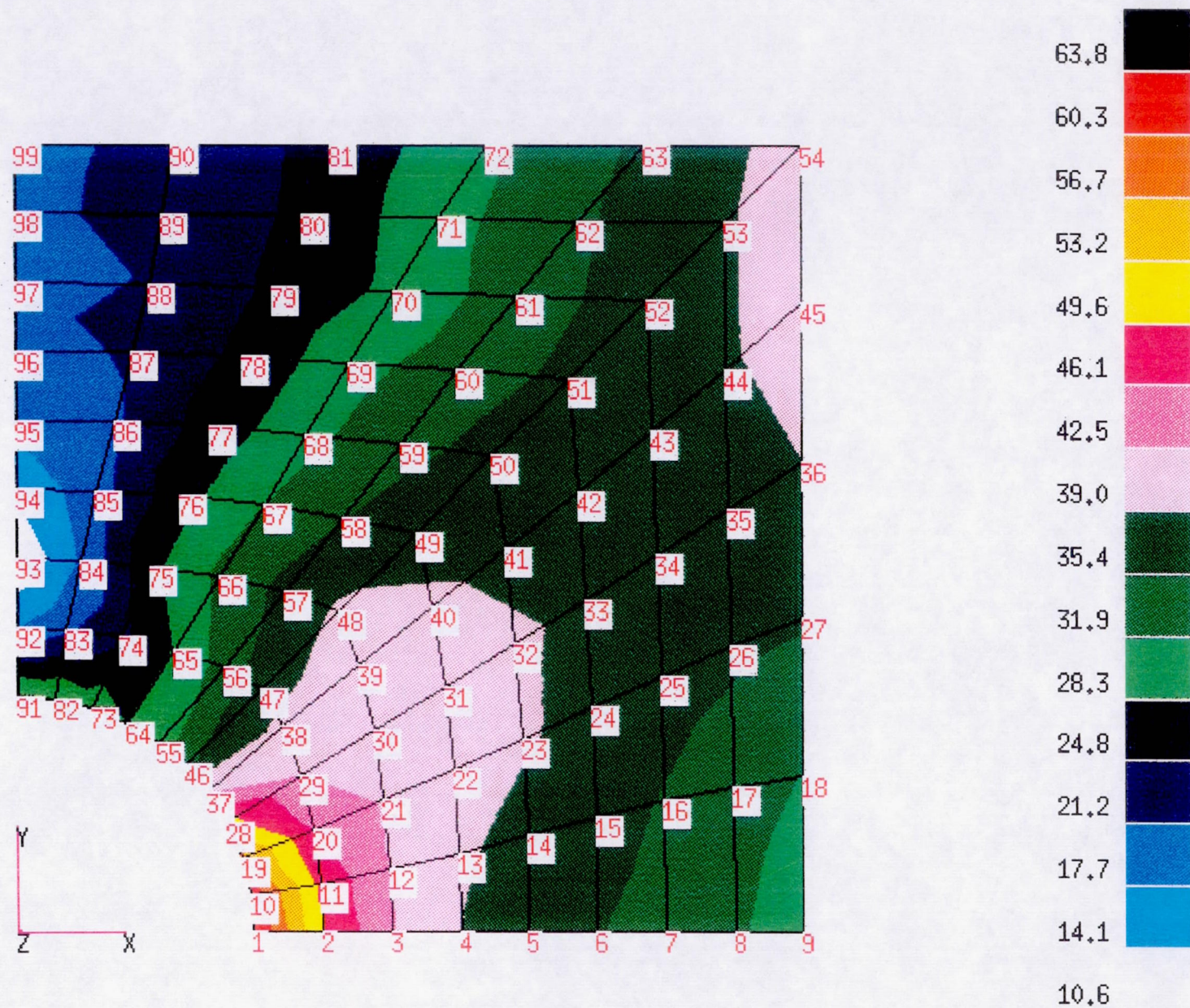
Figure 17 Effective stress distribution (1 step)
