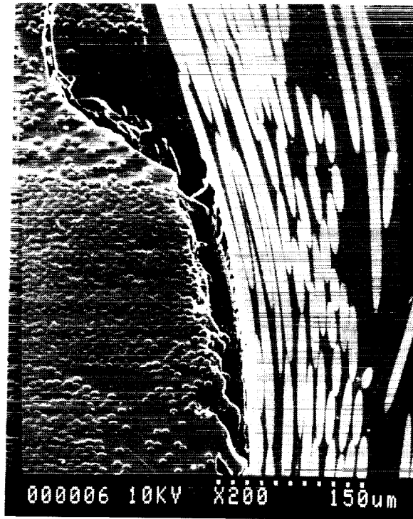
Figure 3. Resin Cavities at Thread
