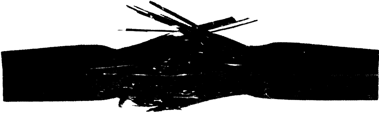
Brooming Failure of Toughened Resin and High Strength Fibers (Prepreg Panel-Unstitched)
