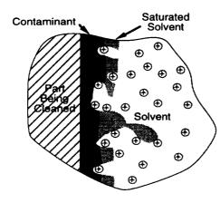
Ultrasonic cavitation and implosion effectively displace the saturated solvent layer to allow fresh solvent to come into contact with the contaminant remaining to be removed. This is especially beneficial when irregular surfaces or internal passageways are to be cleaned.
