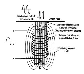
Because of inherent mechanical constraints on the physical size of the hardware as well as electrical and magnetic complications, high power magnetostrictive transducers seldom operate at frequencies much above 20 kilohertz. Piezoelectric transducers, on the other hand, can easily operate well into the megahertz range.
