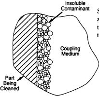
Some contaminants are comprised of insoluble particles loosly attached and held in place by ionic or cohesive forces. These particles need only be displaced sufficiently to break the attractive forces to be removed.
