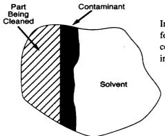
In removing a contaminant by dissolution, it is necessary for the solvent to come into contact with and dissolve the contaminant. The cleaning activity takes place only at the interface between the solvent and the contaminant.
