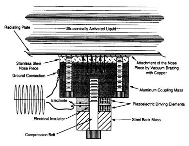
Today's incorporate stronger, more efficient and highly stable ceramic piezoelectric materials which were a result of the efforts of the US Navy and its research to develop advanced sonar transponders in the 1940's. The vast majority of transducers used today for ultrasonic cleaning utilize the piezoelectric effect, and its research to develop advanced sonar transponders in the 1940's. The vast majority of transducers used today for ultrasonic cleaning utilize the piezoelectric effect.
