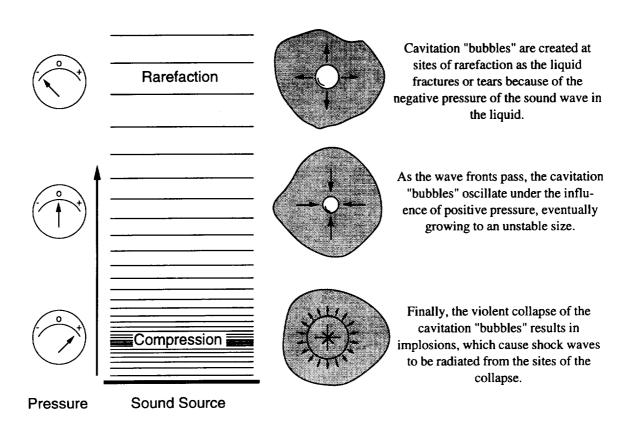
The collapse and implosion of myriad cavitation "bubbles" throughout an ultrasonically activated liquid result in the effect commonly associated with ultrasonics. It has been calculated that temperatures in excess of 10,000°F and pressures in excess of 10,000 PSI are generated at the implosion sites of cavitation bubbles.
