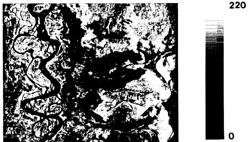
Figure 4: Estimated forest biomass (metric tons/ha) using P-band data in slant range geometry
