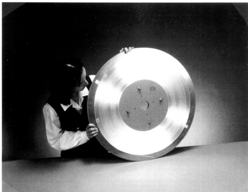
Figure 4.- 61-multifilamentary long high T c superconducting wire.
