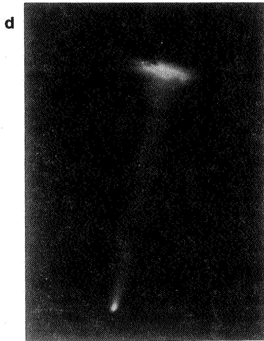
Figure 3. (c) p < 70 mb, discharges with spread-out, blue, diffuse tops. The ionospheric plate is located at the very top of each photograph. Discharge for reverse polarity of the electrodes is shown in (d), which does not resemble jet discharge.
