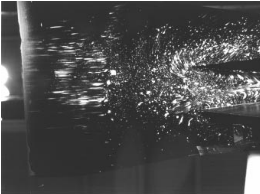
(d) Baseplate, showing oil streaks exiting front of inlet and spilling around sidewalls. CR = 9.
