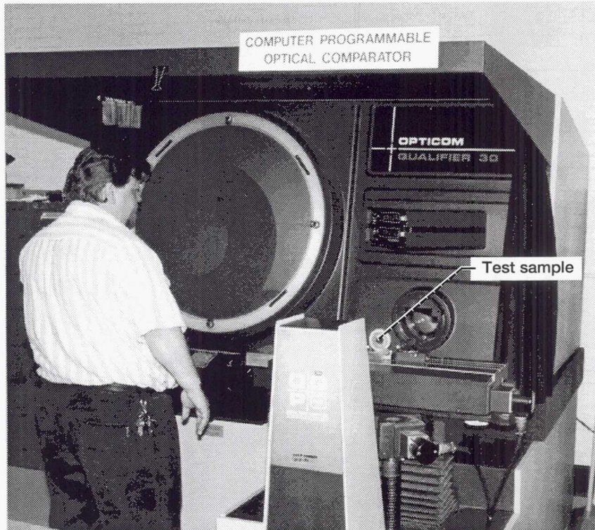
Figure 10.—Optical measurement of test sample.
