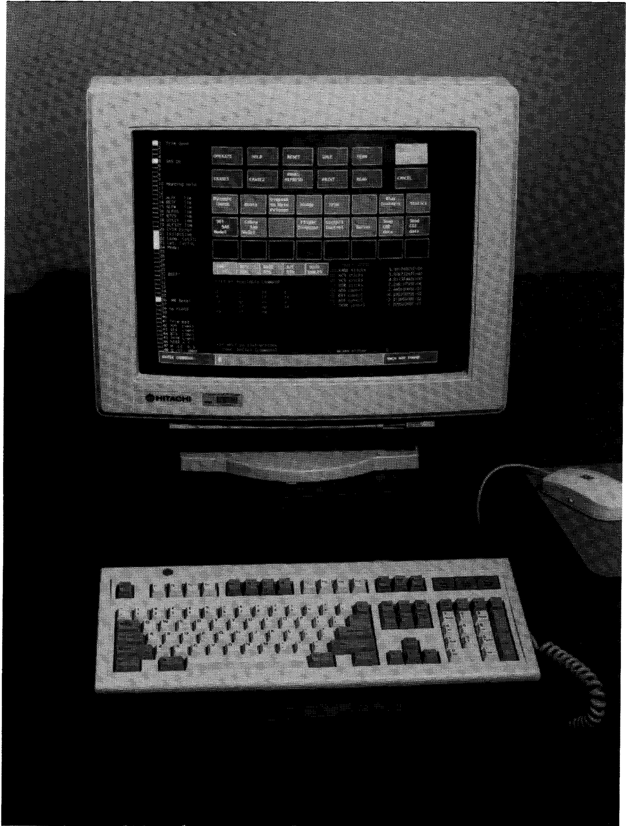
Figure 5. Real-time system console PC.
