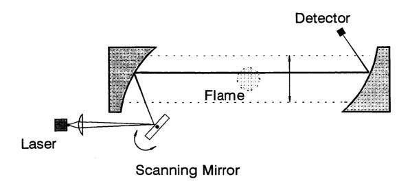
Figure 1 - Schematic of Optical Setup.
