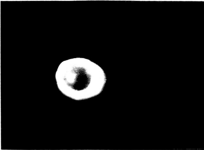
Photo E1. Ethylene flame at 0.067 sec \mu g time. (Flow rate: 20 ml/sec)
