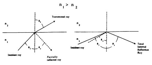
The transmitted ray is bent away from the normal Total internal reflection:  $\theta_i > \theta_c$
