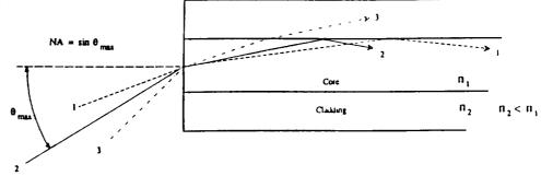
Ray 1: Light is coupled into fiber since ray is within acceptance cone of fiber.
