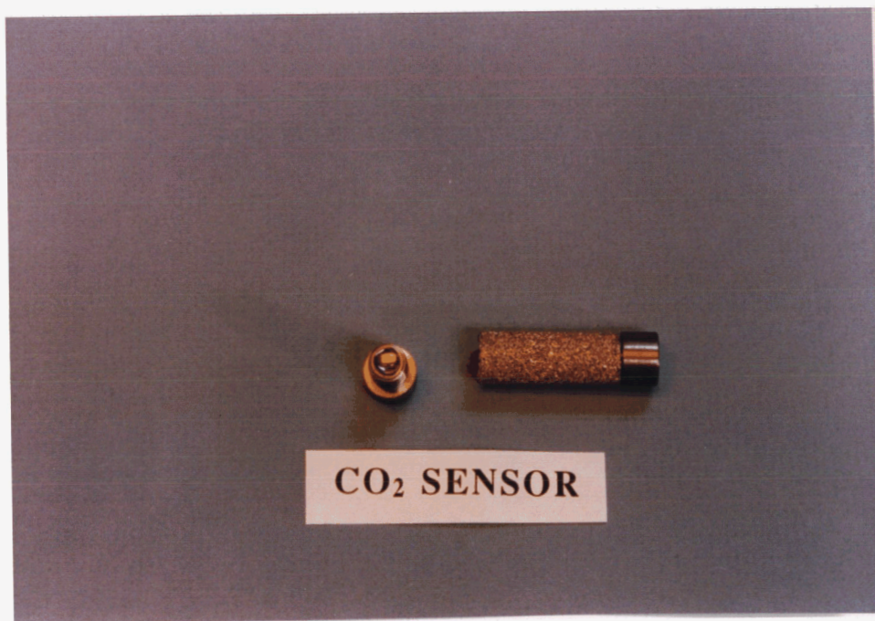
Figure 3-15 Carbon dioxide optrode assembly. A mirror was mounted on a threaded nut (left). The indicator chemistry was spin-coated on the mirror. The threaded nut along with mirror is fitted to the porous metal housing.
