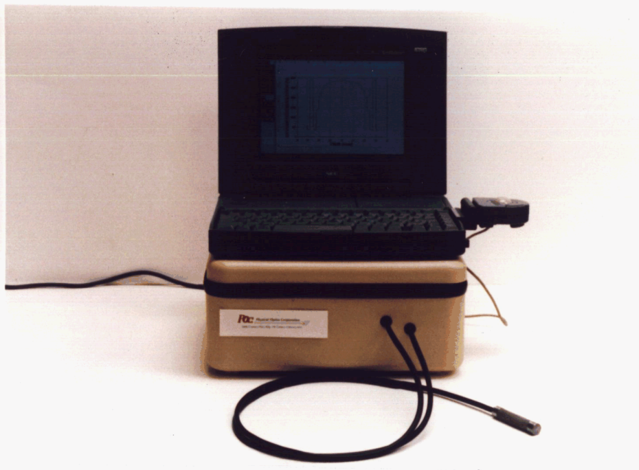
Figure 2-2 POC phase fluorometer, field-ready. The O 2 optrode/cable assembly is also shown.
