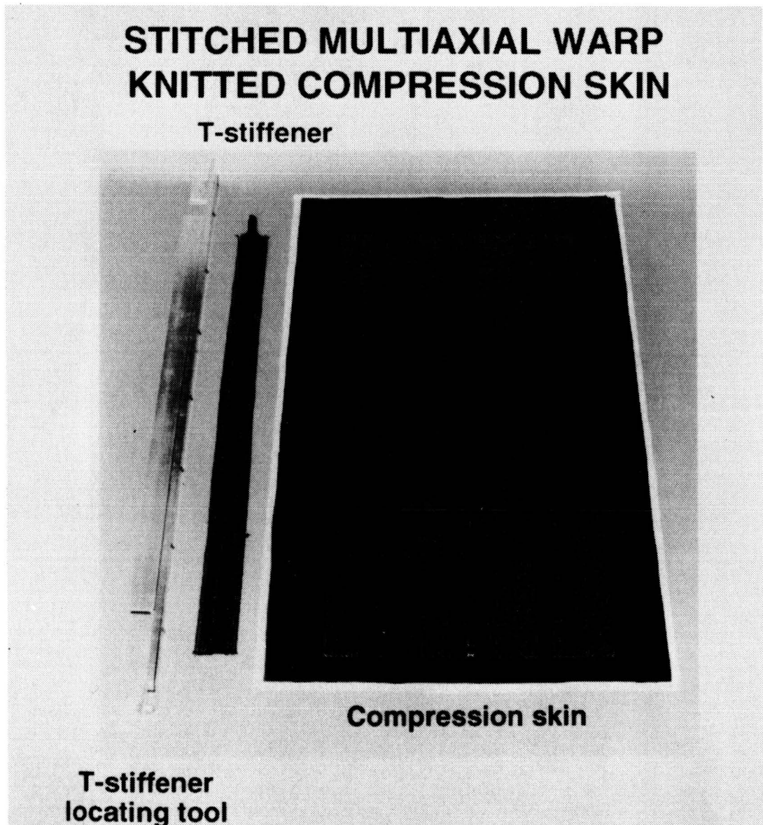
Figure 8. Stitched multi-axial warp knitted compression skin.
