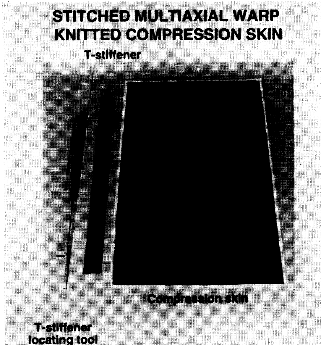
Figure 8. Stitched multi-axial warp knitted compression skin.
