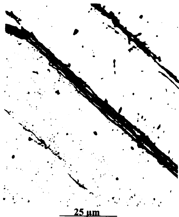
Figure 4.- Optical micrographs of 2195 Al-Li alloy subjected to deformation.
