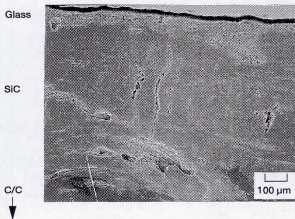
Figure 1.—Electron micrograph of a polished cross section of the oxidation protected RCC material.
