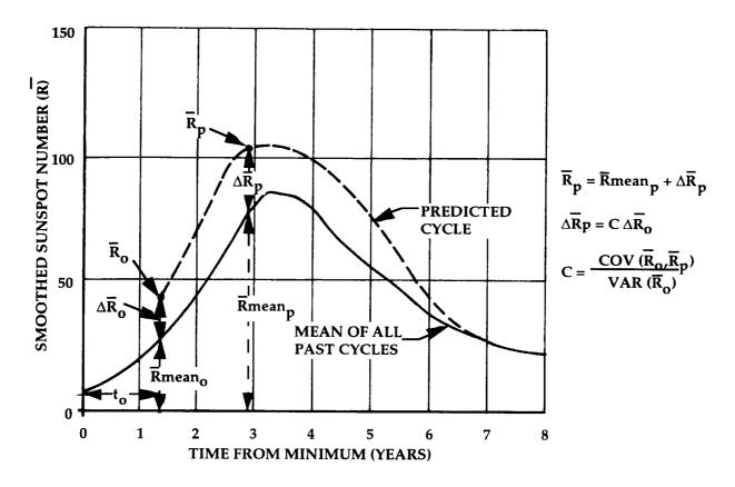
Figure 2-1. Modified McNish-Lincoln Linear Regression Method.
