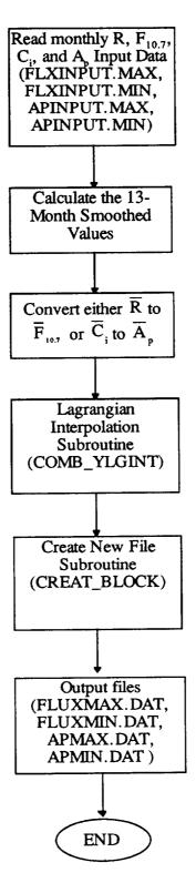
Figure 4-2.  $\overline{F}_{10.7}$  and  $\overline{A}_{p}$  Preprocessor Computer Program Block Diagram.
