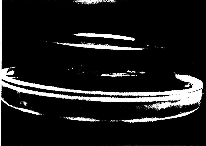
Figure 1. A ring magnet is suspended above a group of large domain levitators.
