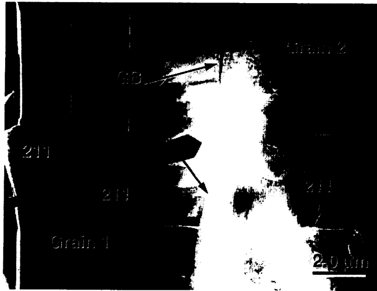
Figure 10. Transmission electron micrograph of two domains with both [001] axes lying in the plane of the paper.
