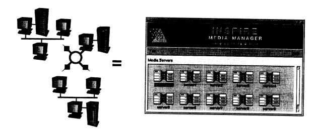
Figure 2. Creating a "virtual single storage environment" from multiple, distributed physical systems using storage fault tolerant software
