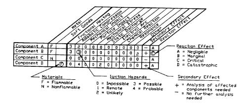
Figure 2 Oxygen Hazards Analysis Chart.
