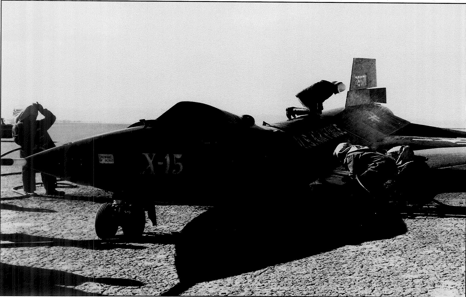
X-15 after a hard landing on the lakebed by Scott Crossfield. On 5 November 1959, the aircraft experienced a small engine fire—a dangerous occurrence in a rocket plane. Crossfield made an emergency landing on Rosamond Dry Lake with a large quantity of propellants still on board. This caused the “back” of the X-15 to break, requiring three months of repairs without significantly delaying the program. (NASA Photo E 9543)
