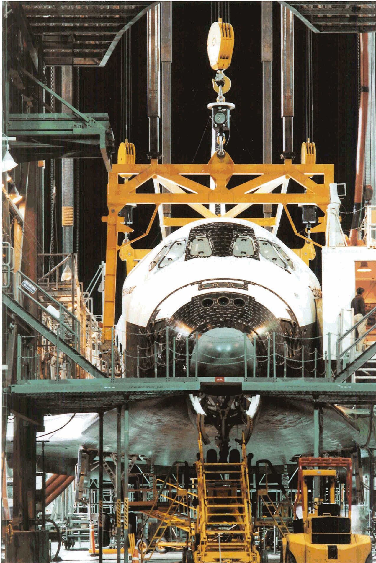
Shuttle mate/demate facility with Space Shuttle Endeavour in it. Endeavour had just completed its first flight (STS-49) from 7 May 1992 to 16 May 1992, when this photo was taken. (NASA Photo EC92 05169-1)
