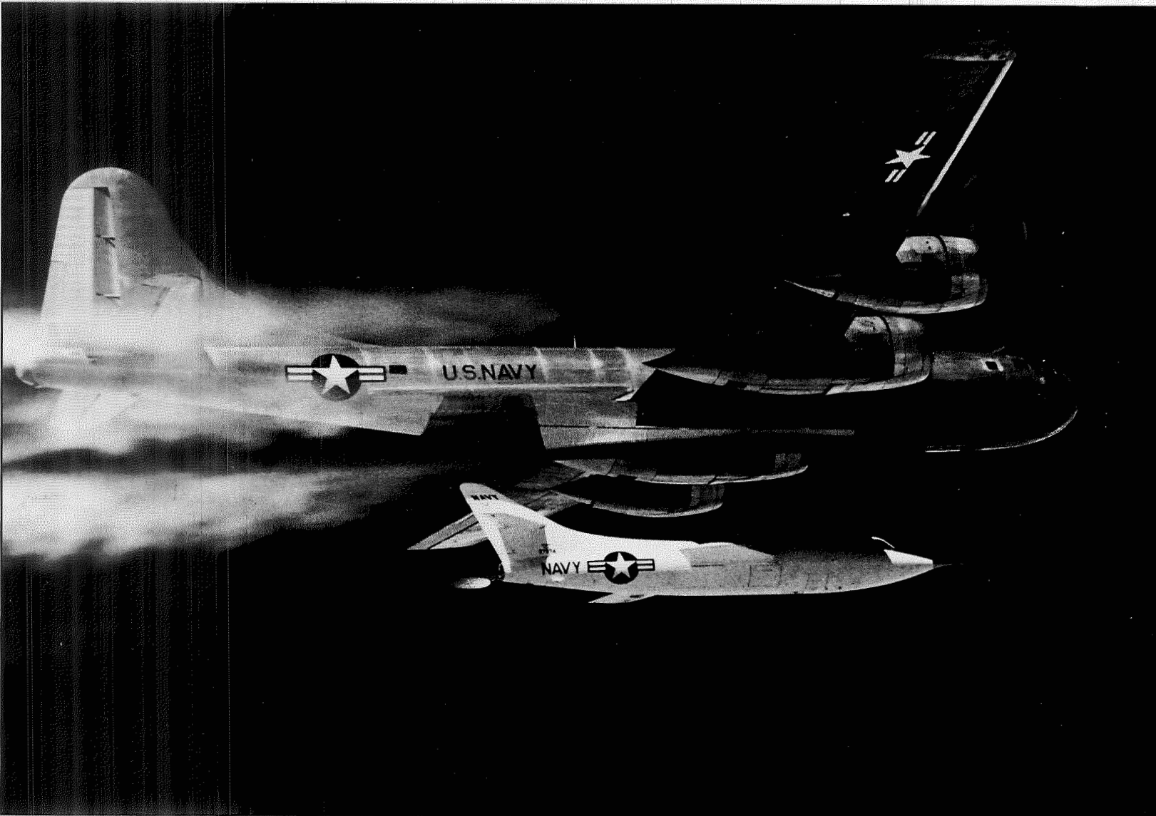
D-558-2 dropping at launch from B-29 mothership (Navy designation: P2B) (NASA Photo E 2478)
