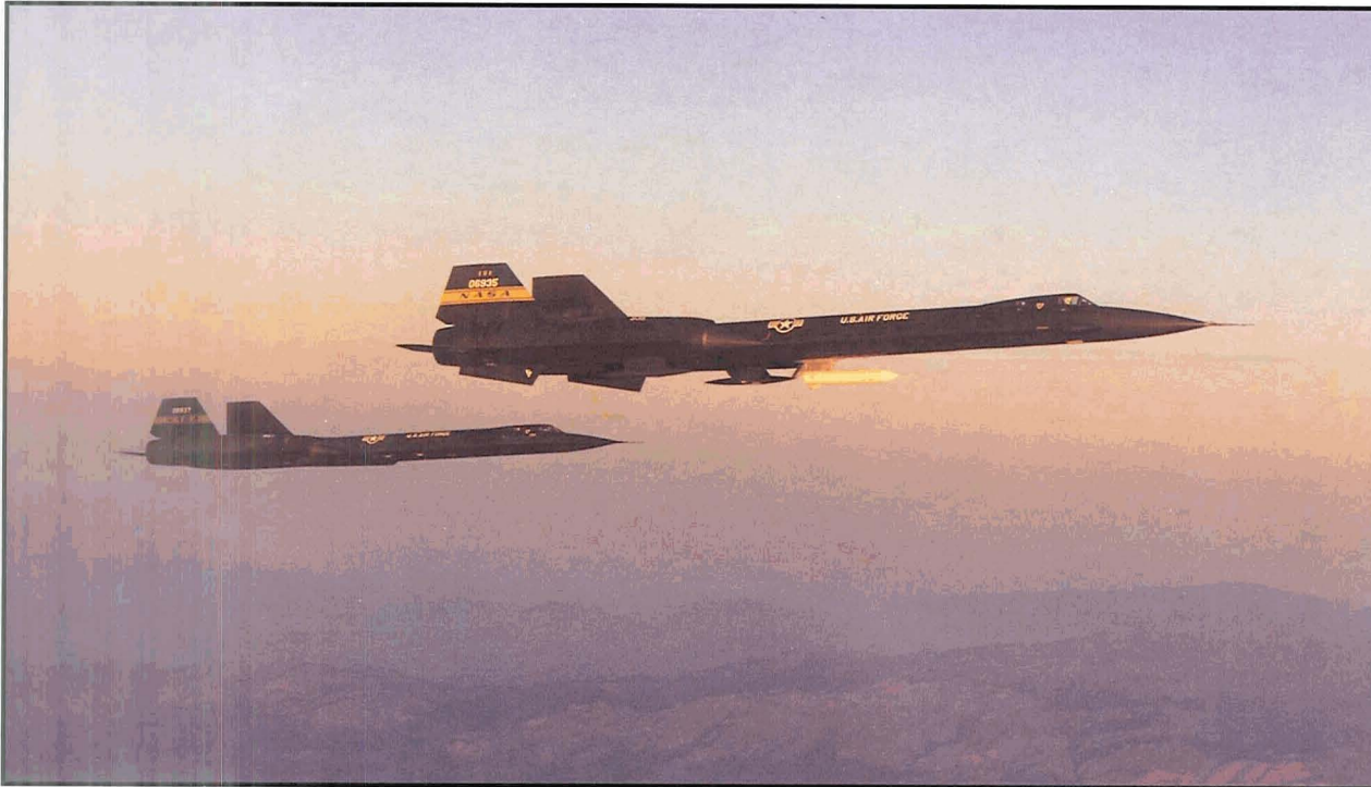
YF-12A (06935) and YF-12C (06937) in formation at dusk, showing the insulated cylinder beneath the YF-12A that was used in the "Cold-Wall Experiment." (NASA Photo ECN 4767)
