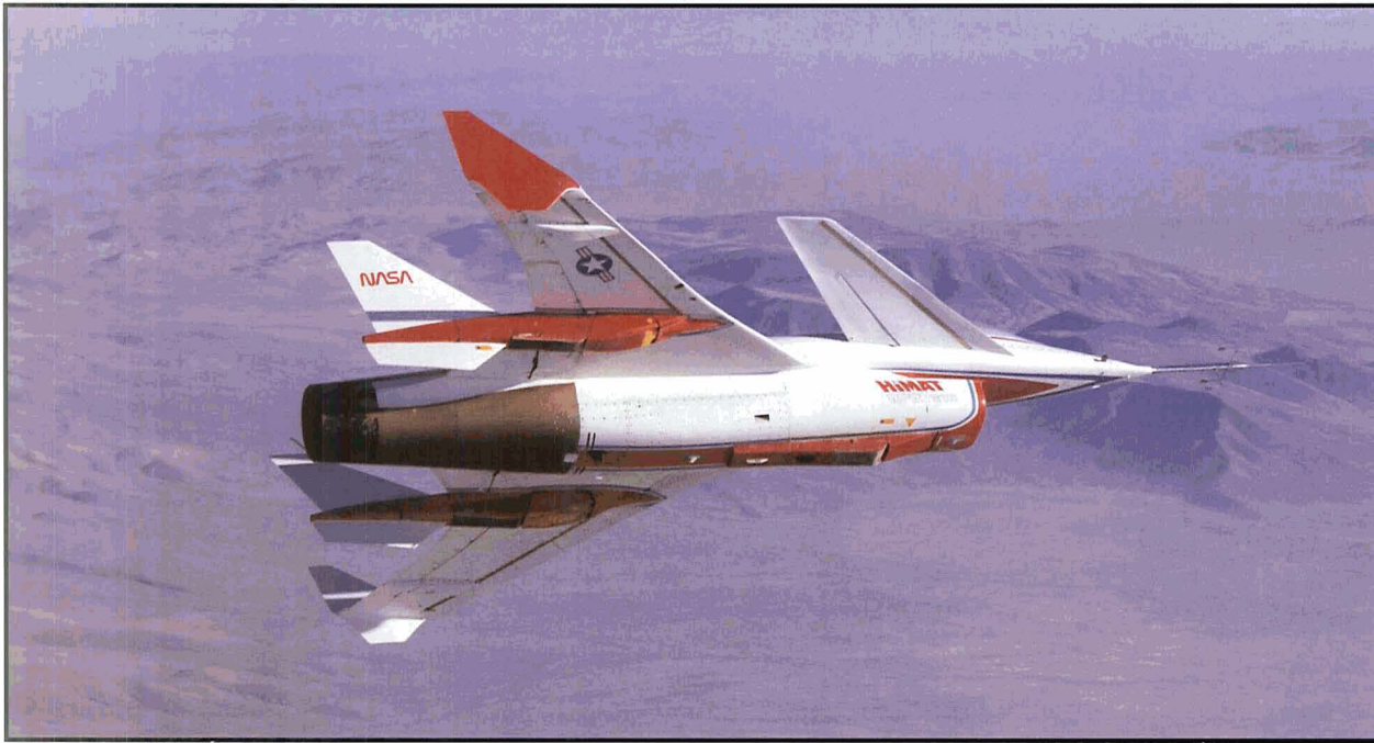
HiMAT (Highly Maneuverable Aircraft Technology) remotely piloted vehicle in flight (NASA Photo ECN 14281)
