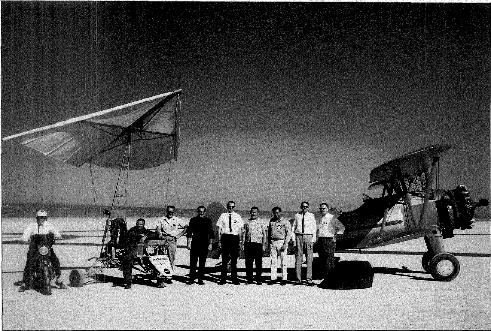
Paresev and crew with one of its tow aircraft, a Stearman biplane, on lakebed; Milt Thompson seated in Paresev and, to his right, a motorcycle with driver who served as the chase observer during lift-off and low-level flights. (NASA Photo E 8713)
