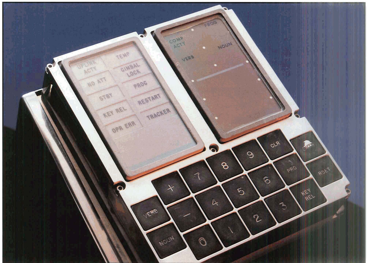
Apollo computer interface box used in the first phase of the F-8 Digital Fly-By-Wire program (NASA Photo EC96 43408-1)
