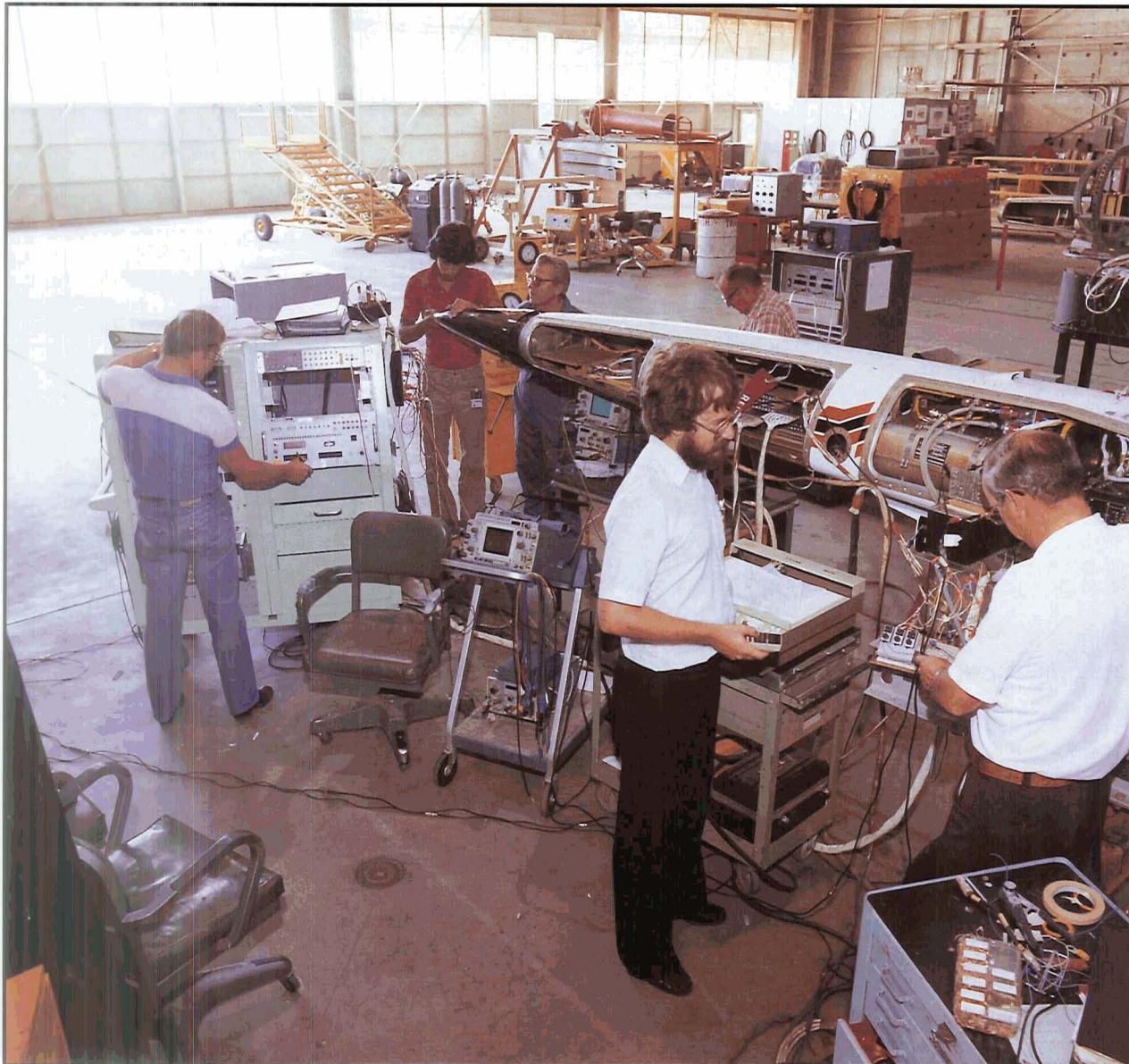
The DAST (Drones for Aerodynamic and Structural Testing) being calibrated in a hangar. The DAST was one of many remotely piloted vehicles used in Dryden research programs because they provide a safer way of obtaining data in high-risk situations than do piloted vehicles. (NASA Photo ECN 20288)
