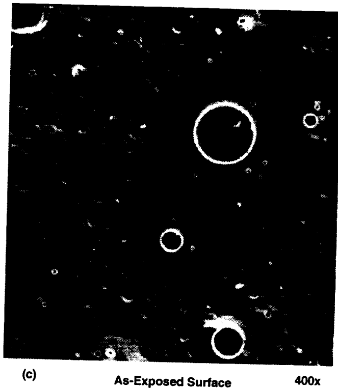
Figure 27. Typical RBN104 Specimen Failure Origins And Surface Topography Following 1050 Hours Exposure At 1371C (2500F).
