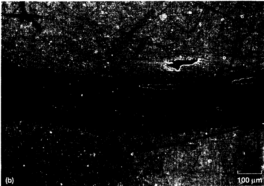
Figure 11.—Wear tracks produced on laser-annealed WS_2 coating after sliding contact. (a) Scanning electron microscopy (SEM) image of wear track and its surroundings at 25 500 passes in air. (b) SEM image of wear track and its surroundings at 2 million passes in dry nitrogen. (c) SEM image of a wear track and its surroundings at 607 990 passes in ultrahigh vacuum.
