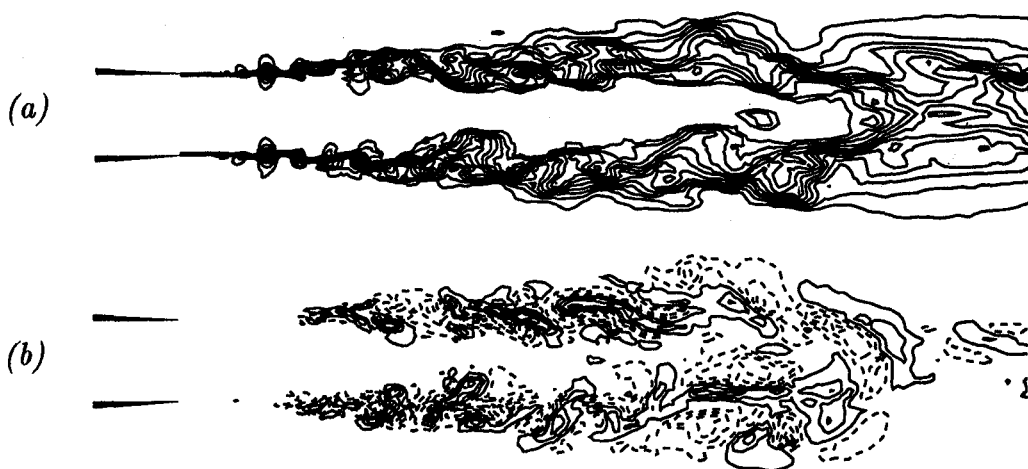
FIGURE 5. Instantaneous planar view of the jet ( \phi = 0 ) at t = 12.1 . The scale can be inferred from the nozzle, which is drawn on the left. The present section is 10 diameters long. (a) Streamwise velocity, with contours drawn from 0.1 to 1.3 in increments of 0.1; (b) azimuthal velocity, with contours drawn from -0.45 to 0.45 in increments of 0.1. Dotted contours indicate negative values.
