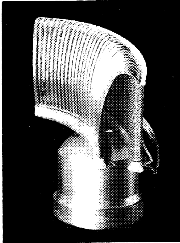
Figure 3-5. Typical Annular Heater Head
