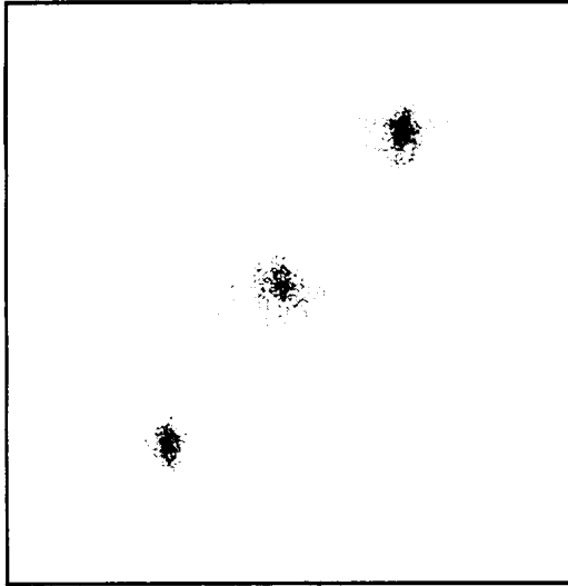
Figure 1 Images of three 10\mu\text{m} pinholes obtained with a 10\mu\text{m} pore MCP Z stack and a 90\text{mm} \times 15\text{mm} HDDL anode readout.
