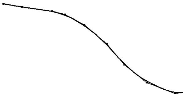
Figure 3.31 An interpolated BSpline curve for nozzle boundary.
