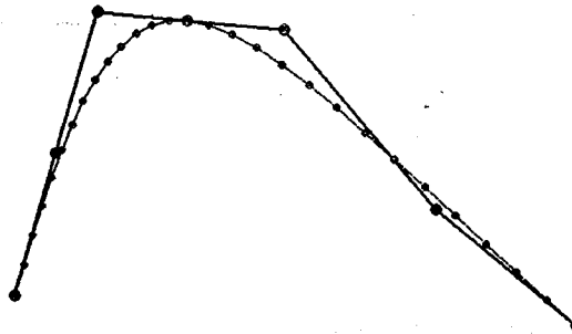
Figure 2.7 BSpline control polygon for parametric curve with 2 segments.
