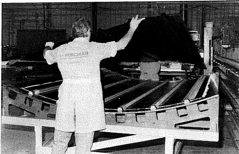
Figure 3-47. Locating Stringers with IML Cauls
