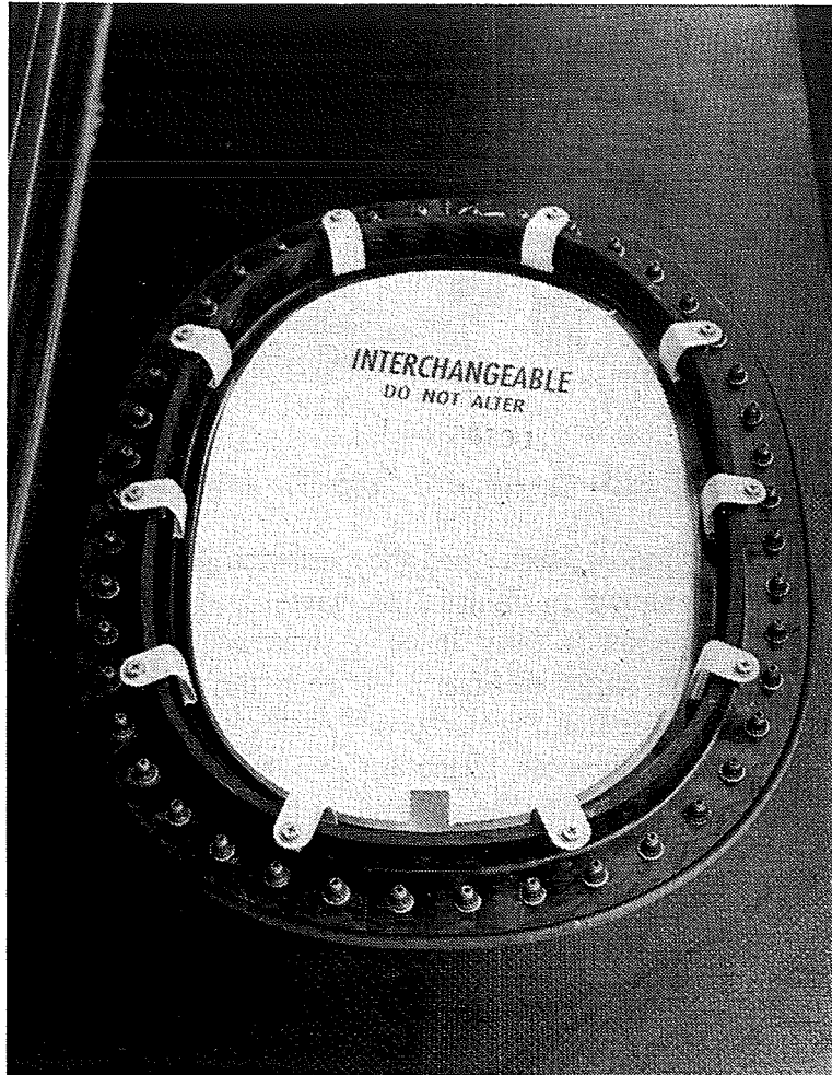
Figure 5-42. Window Frame Element Installed and Assembled
