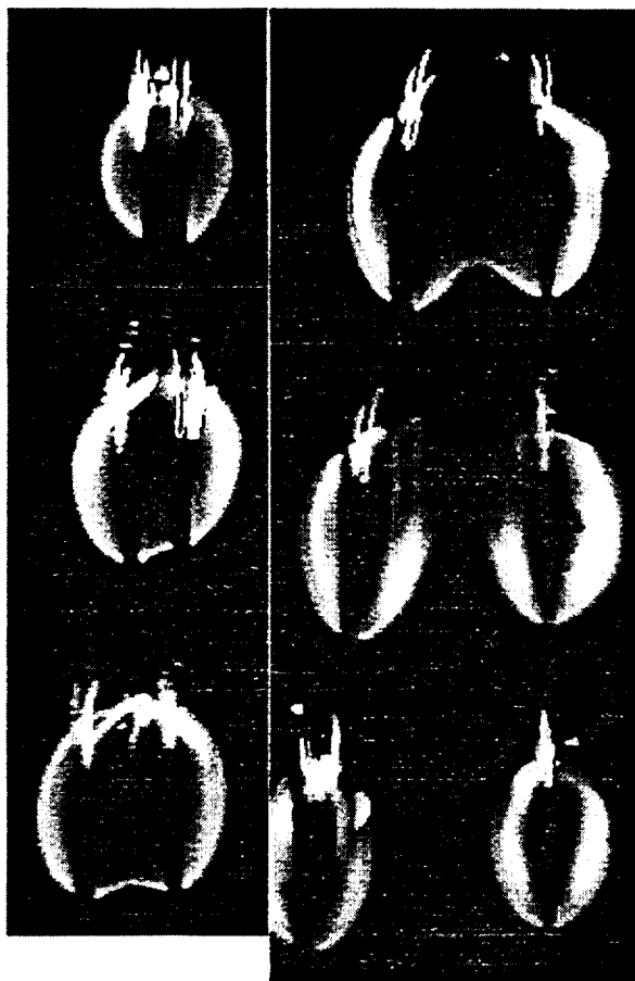
Figure 4. Edge view of flames propagating in microgravity over parallel sheets of Kimwipe at different separation distances in 30% oxygen, balance nitrogen, at 1 Atm. Separation distances in order (top to bottom, left to right) are 6.4, 10, 20, 30, 40 and 50 mm. Glowing material at top of each flame is the ignitor wire.
