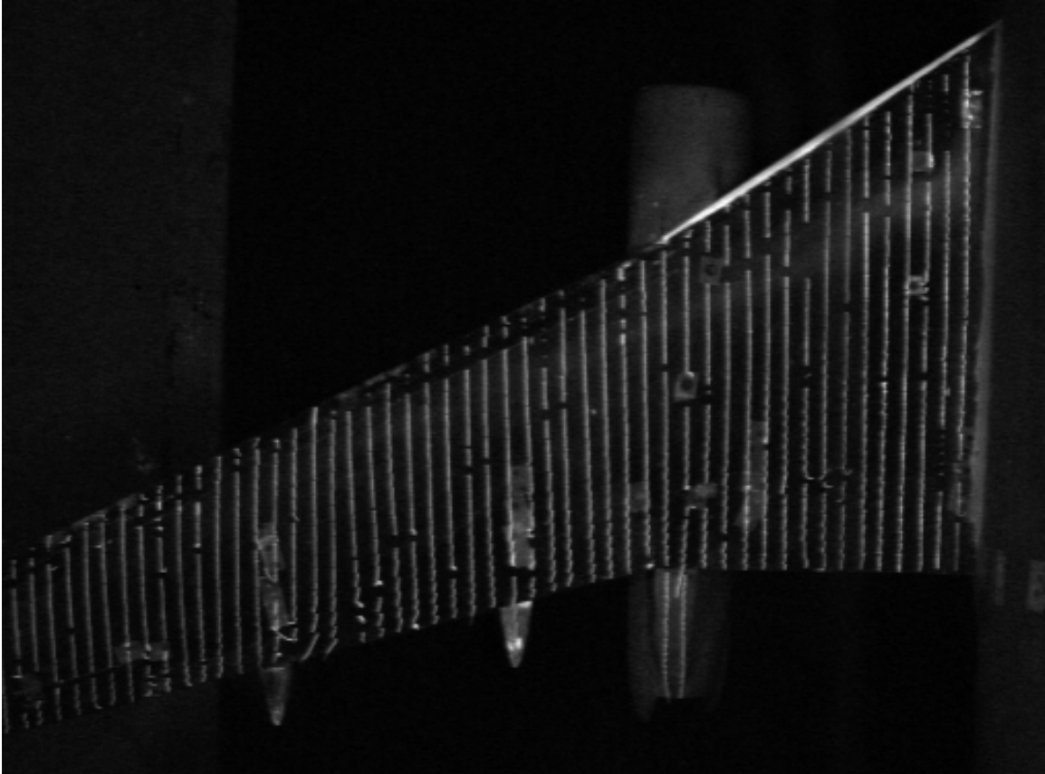
Figure 81.—Wing mini-tuft flow visualization for inboard wing ice #1, cruise configuration, \alpha = 4^\circ , run 481 condition.
