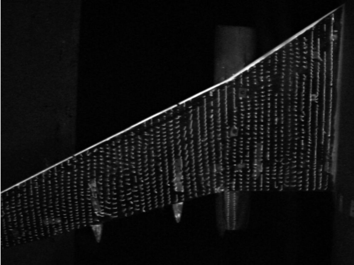
Figure 77.—Wing mini-tuft flow visualization for all wing ice #1, cruise configuration, \alpha = 14^\circ , run 464 condition.
