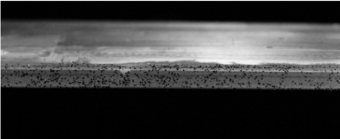
Figure 4.—Grit applied to ice shapes.
