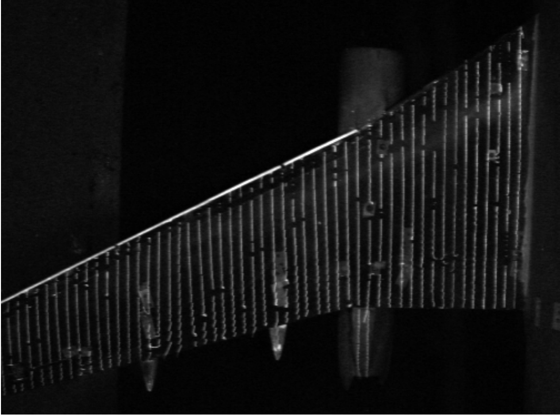
Figure 78.—Wing mini-tuft flow visualization for outboard wing ice #1, cruise configuration, \alpha = 4^\circ , run 474 condition.
