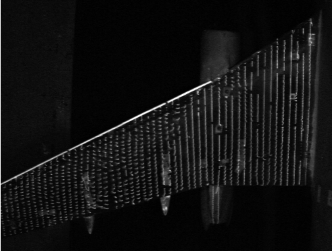
Figure 79.—Wing mini-tuft flow visualization for outboard wing ice #1, cruise configuration, \alpha = 10^\circ , run 474 condition.
