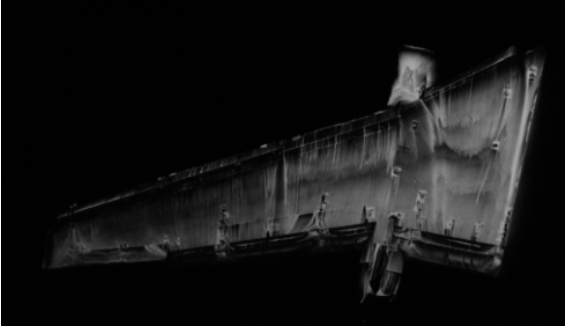
Figure 25.—Main wing flow visualization for no ice, \delta_f=40^\circ , \alpha=10^\circ condition.
