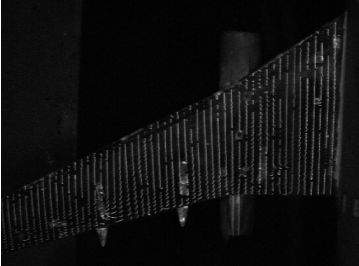
Figure 45.—Wing mini-tuft flow visualization for no ice, cruise configuration, \alpha = 10^\circ , run 500 condition.
