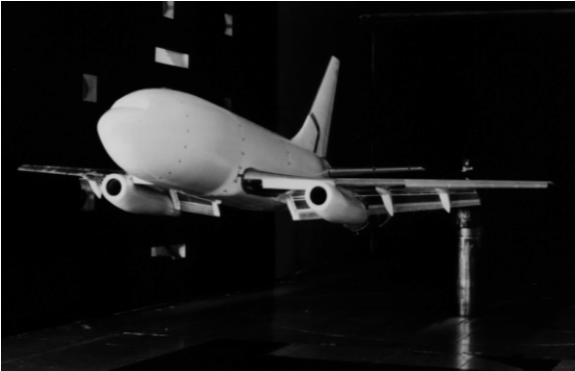
Figure 1.—NASA Langley 1/8 scale twin engine subsonic transport model.
