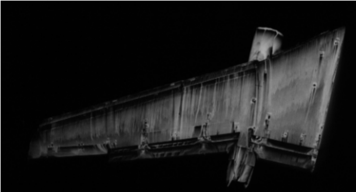
Figure 17.—Main wing flow visualization for ice #2, \delta_f=40^\circ , \alpha=0^\circ condition.
