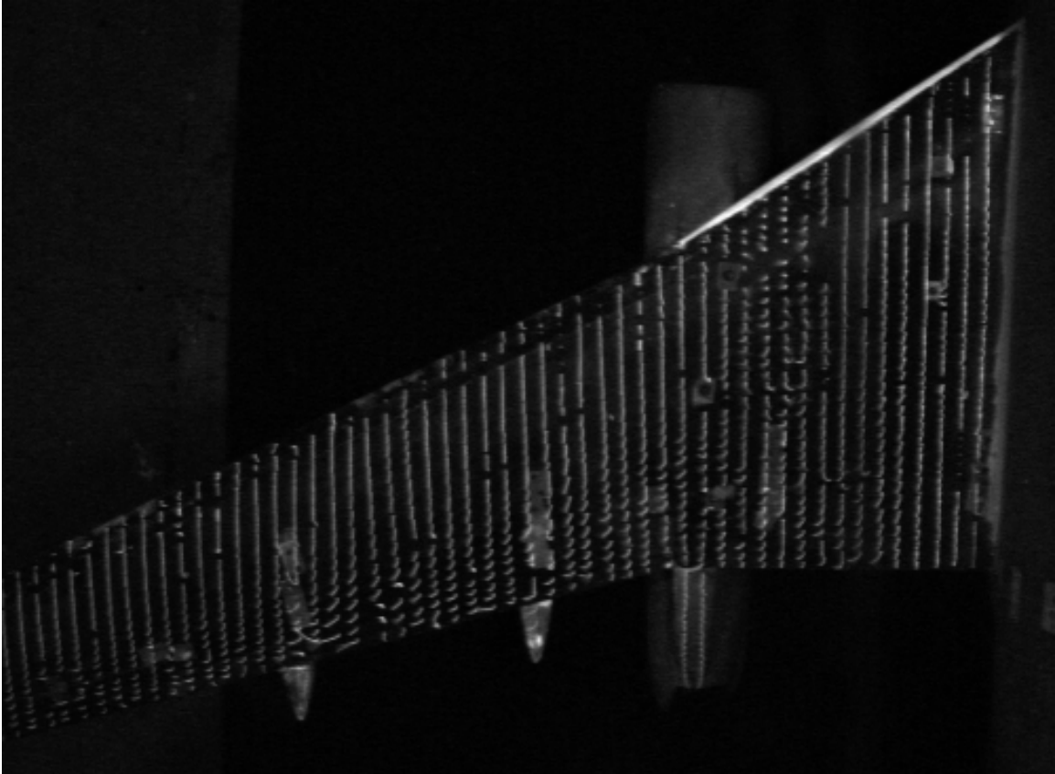
Figure 82.—Wing mini-tuft flow visualization for inboard wing ice #1, cruise configuration, \alpha = 10^\circ , run 481 condition.
