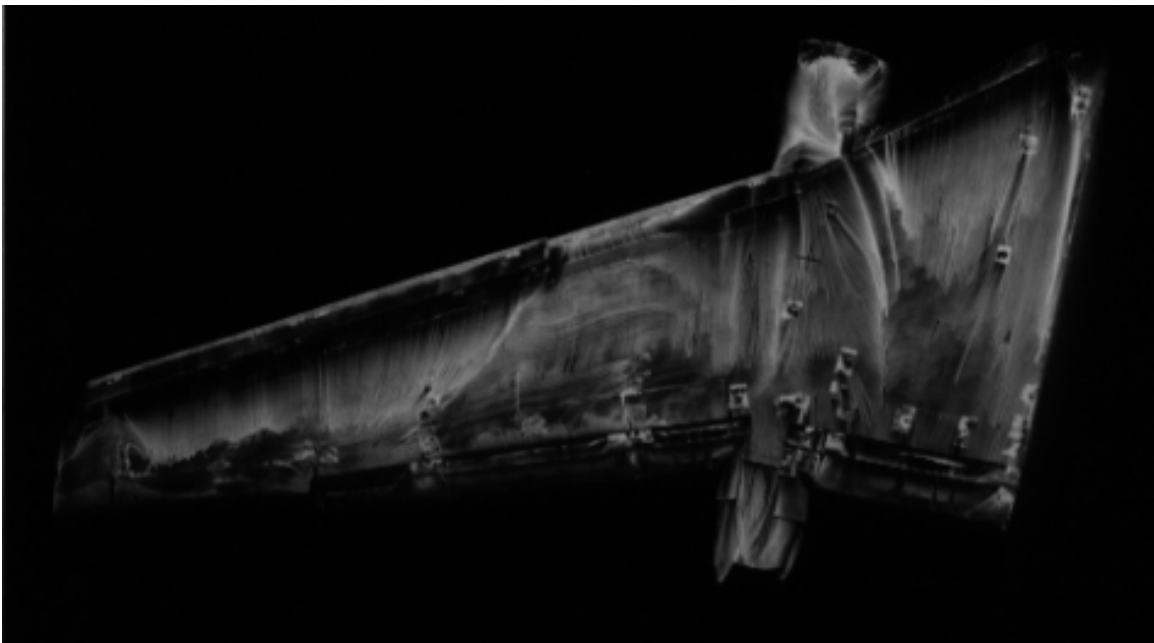
Figure 20.—Main wing flow visualization for ice #2, \delta_f=40^\circ , \alpha=12^\circ condition.
