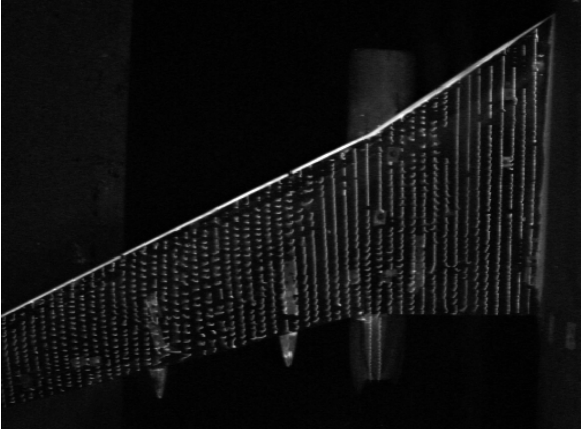
Figure 76.—Wing mini-tuft flow visualization for all wing ice #1, cruise configuration, \alpha = 10^\circ , run 464 condition.
