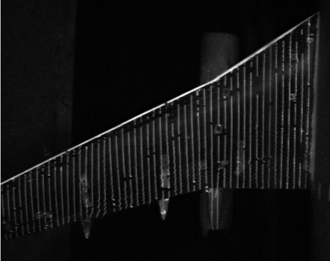
Figure 75.—Wing mini-tuft flow visualization for all wing ice #1, cruise configuration, \alpha=4^\circ , run 464 condition.
