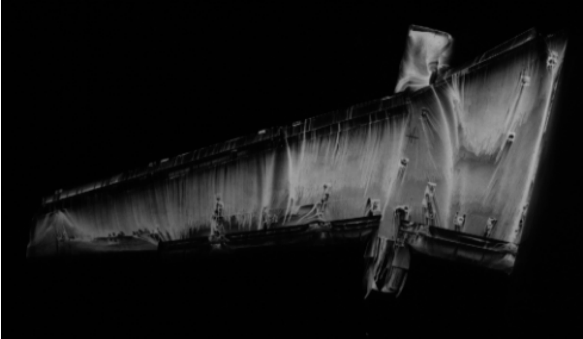
Figure 27.—Main wing flow visualization for no ice, \delta_f=40^\circ , \alpha=13^\circ condition.
