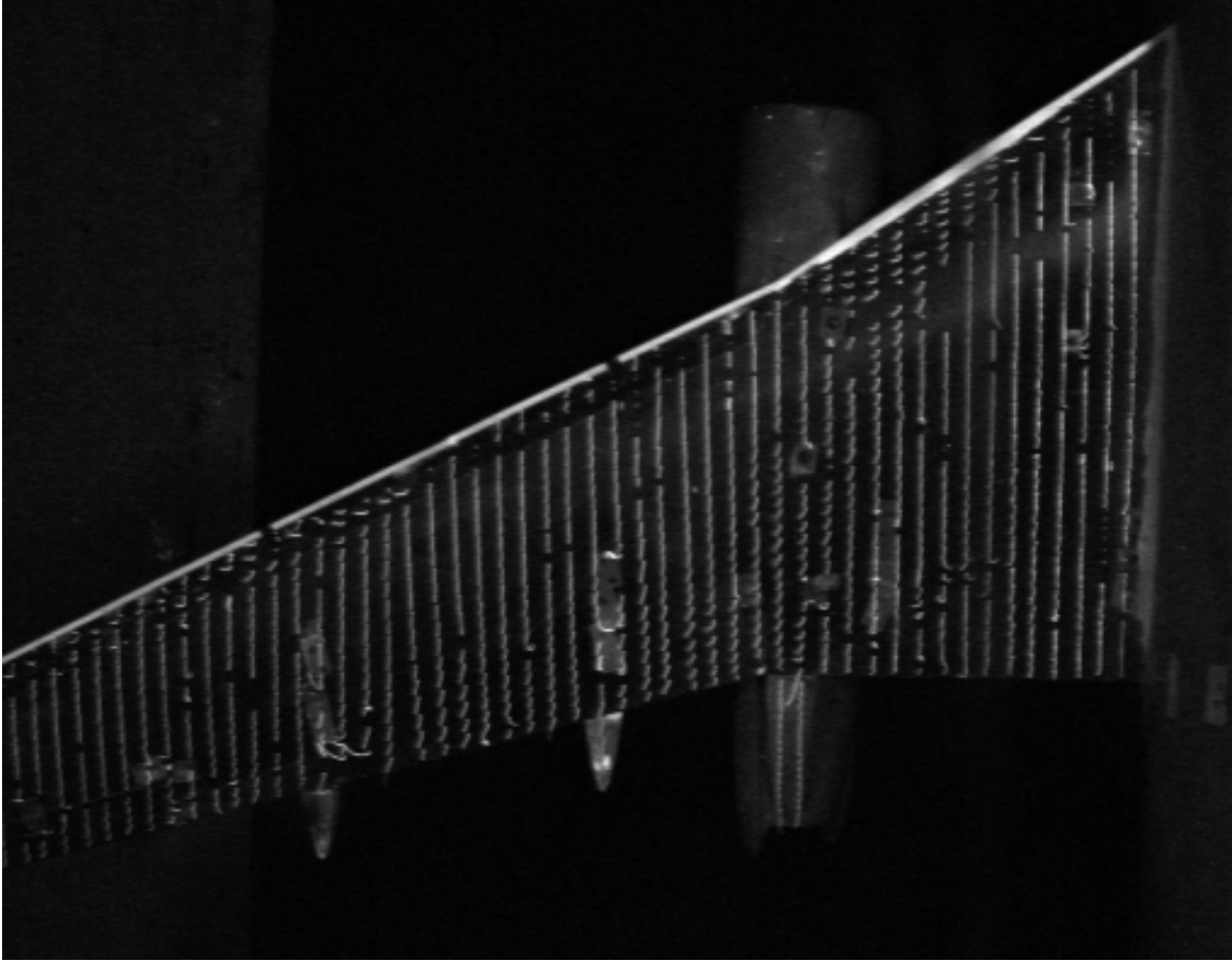
Figure 35.—Wing mini-tuft flow visualization for all wing ice #2, cruise configuration, \alpha=4^\circ , run 495 condition.
