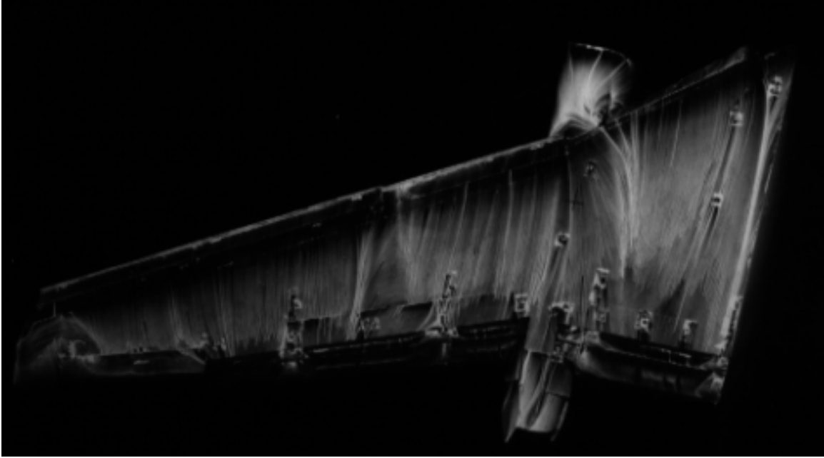
Figure 19.—Main wing flow visualization for ice #2, \delta_f=40^\circ , \alpha=10^\circ condition.
