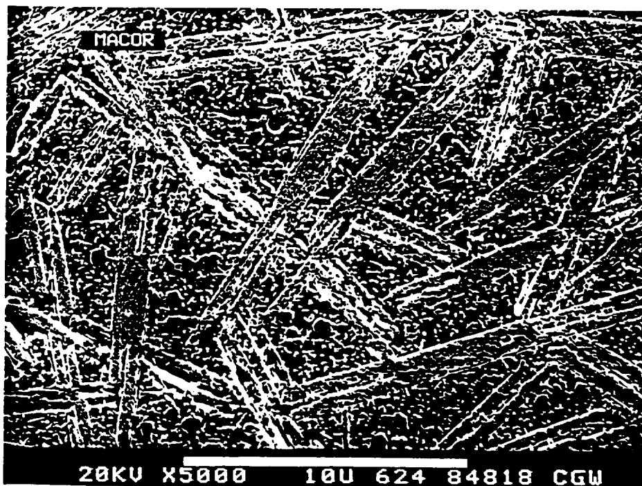
Figure 2: Microstructure of MACOR MGC 5000X magnification.
