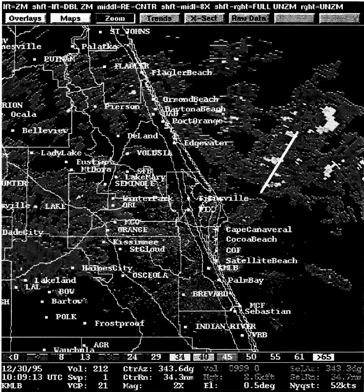
Figure 4.2. WSR-88D base reflectivity image at 1008 UTC. White line marks a cross-section (Figure 4.3).
