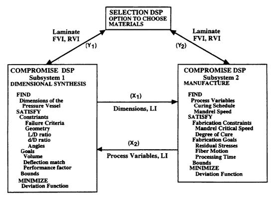
Figure 4.12. Multi-Level Pressure Vessel: Coupled Selection-Compromise DSPs and Interactions
