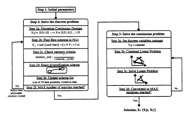
Figure 6.4. Schematic of FALP Solution Scheme
