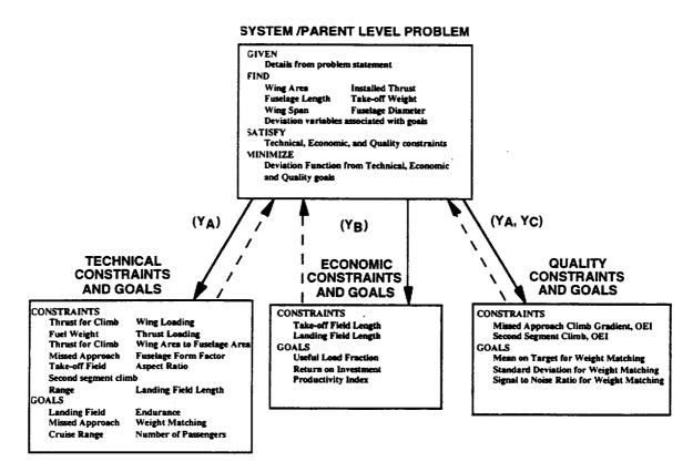
Figure 4.6. Multiobjective Aircraft Compromise DSP
