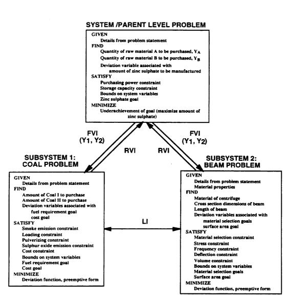
Figure 4.9. Multi-Level Thermal System: Coupled Compromise DSPs and Interactions
