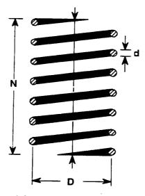
Figure 6.5. Coil Compression Spring
