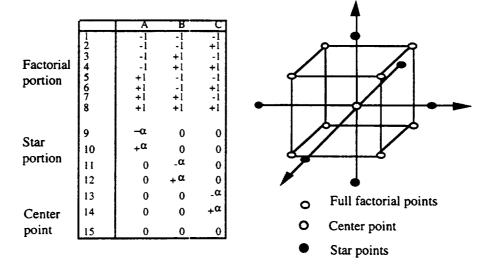
Figure 3.14. Three Variable Central Composite Design
