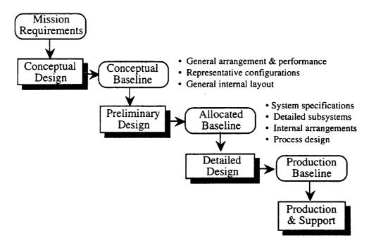
Figure 1.3. Four Phases in Aircraft Design (Schrage, 1992)
