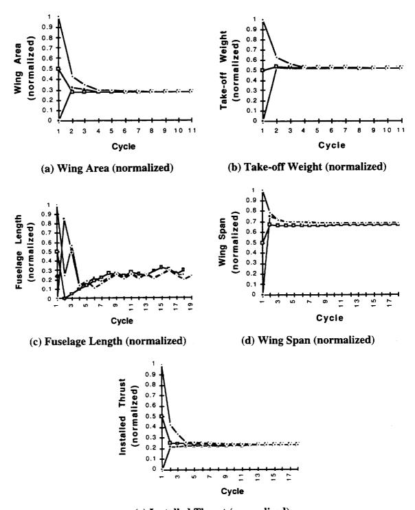
(e) Installed Thrust (normalized) Figure C.4. Design Variable History: Full Cooperation (Continuous)
