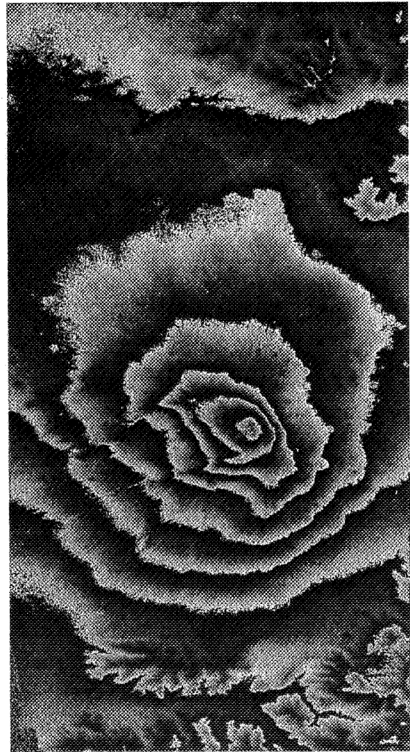
Figure 4 Mt. Etna Flat Terrain subtracted interferogram (SIR-C L band)
