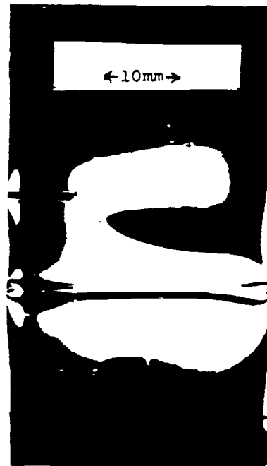
Fig. 4 No-Load Fringe Pattern for B-4 (12.7mm) Data Zone lies between 1.17 and 3.43 mm above crack tip along a reading line inclined 8^\circ to a normal to the crack plane for B-4, 13^\circ for B-5 and 17^\circ for B-6.
