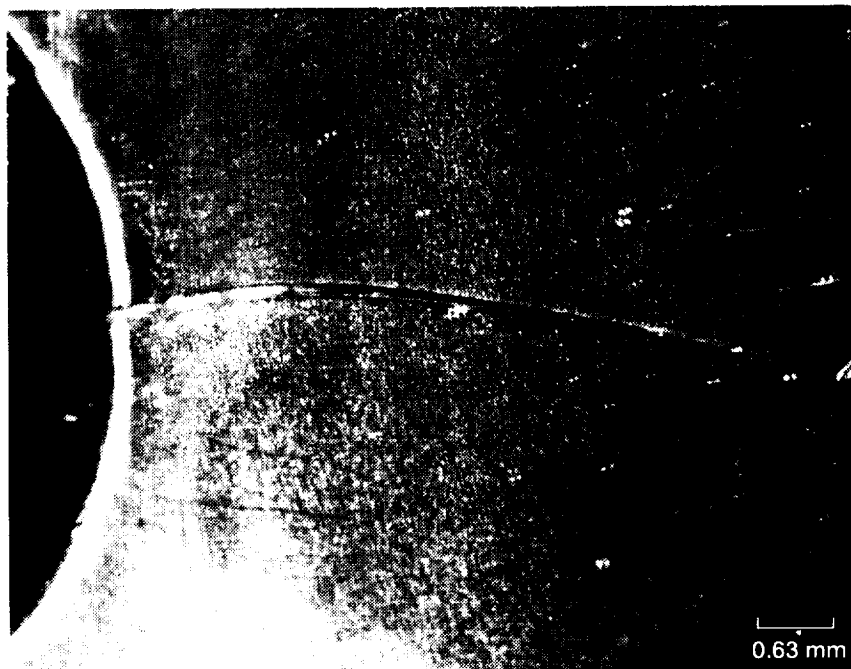
Figure 5. Through-thickness crack in the solar facing side of the HST SADA adjacent to a vent hole.
