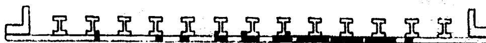
Figure 3. Damage of Skin and Stiffeners at the Doubler Edge on Wing Lower Surface: D16T Alloy; \sigma_{\text{fract net}} = 0.9 \sigma_{0.2} ; K_{\text{fract}} = 0.5 K_c^{\text{app}} .
