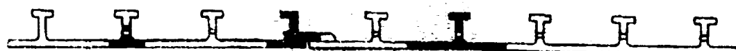
Figure 5. Damage of Skin and Stiffeners on Wing Lower Surface Near Fuel Holes in the Stringers: D16T Alloy; \sigma_{\text{fract net}} = 0.7 \sigma_{0.2} ; K_{\text{fract}} = 0.5 K_c^{\text{app}} .
