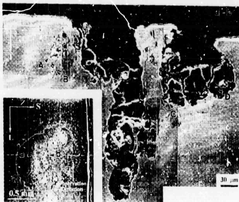
Figure 2. SEM Micrograph of the Cross Section of Severe Corrosion Pits in a 2024-T3 Alloy (TS) Surface With an Inset Showing the Corresponding Surface Appearance of the Pits.
