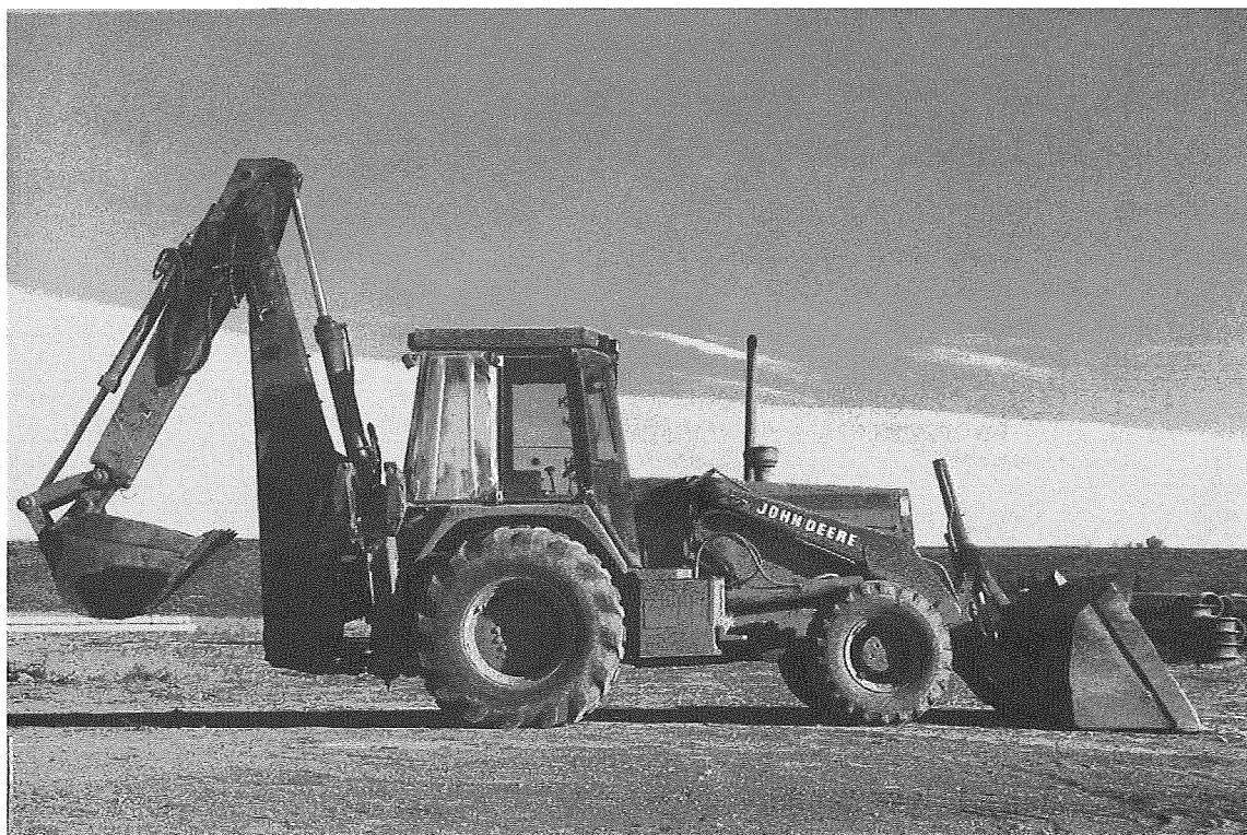
Figure 17. This type of backhoe masses about 450 kg and has a bucket capacity of 0.2 m 3 to 0.3 m 3 .
