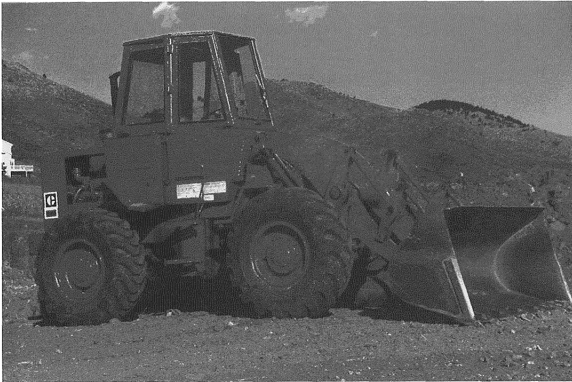
Figure 14. This model of front-end loader has an operating mass of 9,000 kg, a height (with bucket raised) of 4.7 m, a length of 6.6 m, and a width of 2.4 m. Capacity varies from 1.4 m 3 to 1.7 m 3 depending on the bucket configuration (data from Caterpillar [7]).
