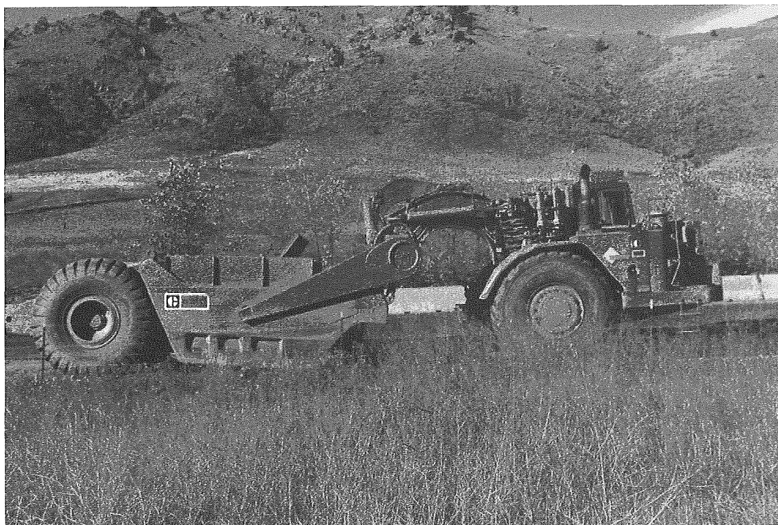
Figure 12. This model of scraper has an operating mass of 44,000 kg, a height of 4.3 m, a length of 14.3 m, and a width of 3.9 m. Machine capacity is 23.7 m 3 (data from Caterpillar [7]).
