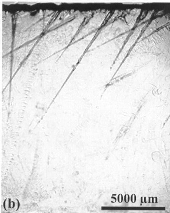
Figure 12a-b. Examples of aerogel penetration tracks produced at variable impact angles. Target (a) was exposed twice, while target (b) was used in three experiments, as can be seen from the variable inclinations of the penetration tracks. Note the overall reproducibility of track length among individual and different experiments in any given aerogel specimen.
