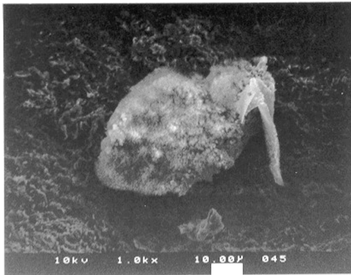
SEM image of Allende projectile recovered from a penetration track into a 20mg/cc AEROGEL target .
