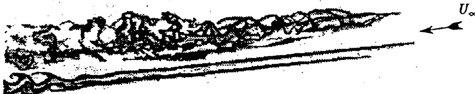
(h) Flow visualization by Stage-smoke method of high frequency secondary instability from diagonally above view and its sketch. (Perspective view, U_\infty=10\text{m/s} , Re_c=5.3 \times 10^5 , nozzle position x/C=0.35 , y = \pm 100\text{mm} )
