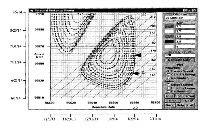
E=Minimum flight time trajectory using 2011 Piloted Mission Departure Excess Speed (3.99 km/sec) and while maintaining acceptable Mars entry velocity needed for aerobraking.
