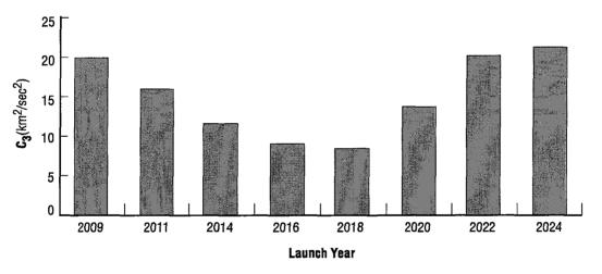
Figure 8. Piloted optimal departure energies, 2009-2024.
