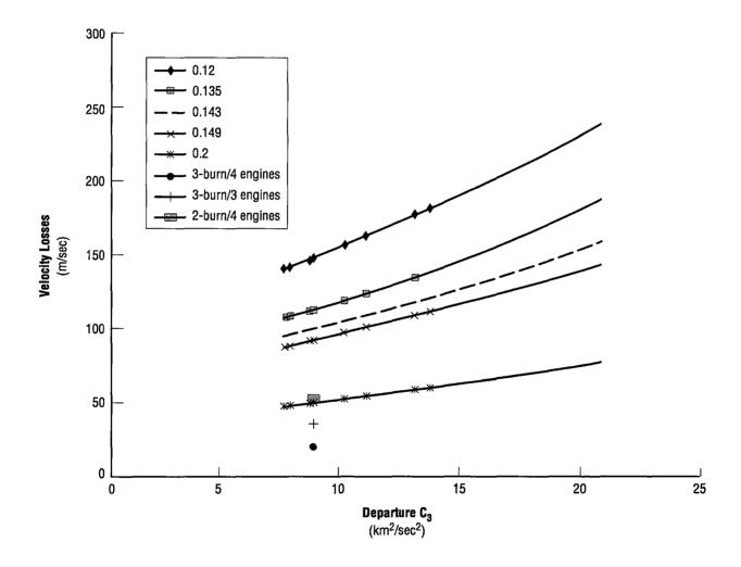
Figure 11. Velocity losses at various T/W ratios.
