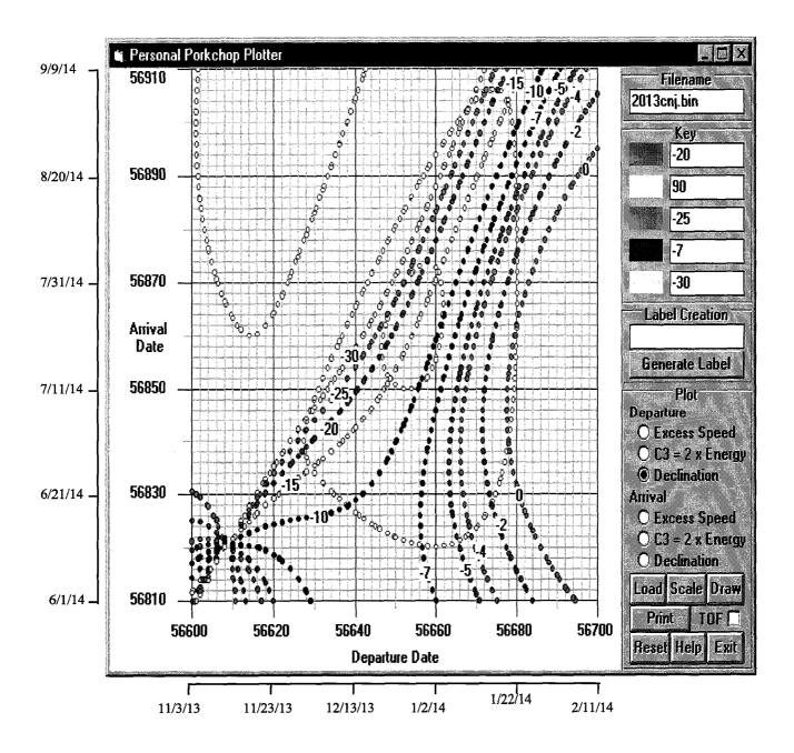
Earth-Mars Trajectories 2013/14 Piloted Missions Baseline Mission Designed to 2011 Departure Excess Speed
