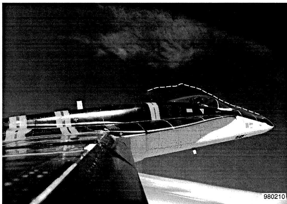
Fig. 7. Forebody/strake vortex flow visualization for \alpha = 50^\circ , \delta_{s,d} \approx 19^\circ , and \delta_{s,L/R} = 0^\circ/19^\circ .
