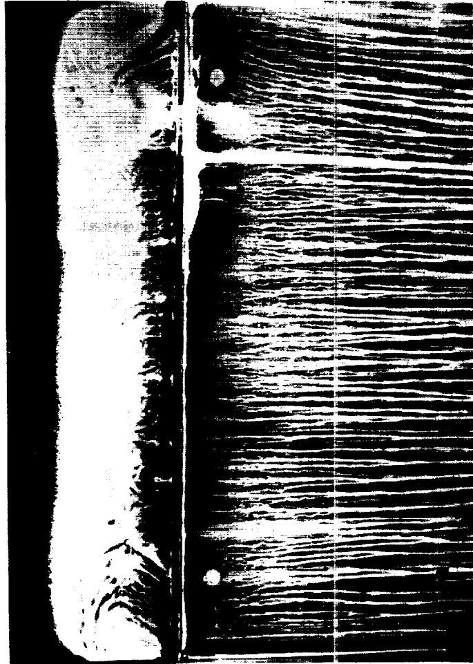
Figure 7.- Smooth-step model ( h = 0 ) with fluorescent-oil coating and wire; h = 0.051 inch, R/l = 7.7 \times 10^6 per foot.
